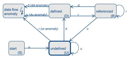
If the state data flow anomaly is reached or at the end of a data flow anomaly analysis the state undefined is not reached, a data flow anomaly is detected. The state machine defines a regular grammar. Such grammars are a standard case for compiler construction. In compilers they serve as a basis for the lexical analysis. Thus, data flow analysis can be integrated into compilers (which is the case in some compilers → you should check whether your compiler can do it)
