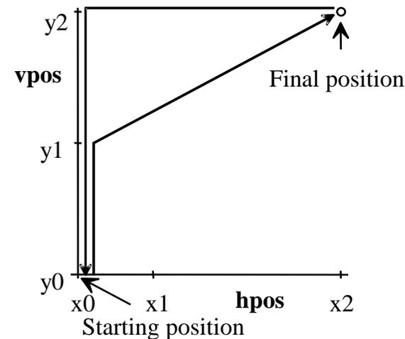
*A safety requirement has to be considered. The table is not allowed to move into the forbidden area. This is ensured, if the states where  $[vpos=y0 \wedge (hpos=x1 \vee hpos=x2)]$  is true are not reachable. For this reason, during the upward movement the horizontal motion is started at the vertical position  $y1$ , and not before. This applies analogously for the downward motion.*
