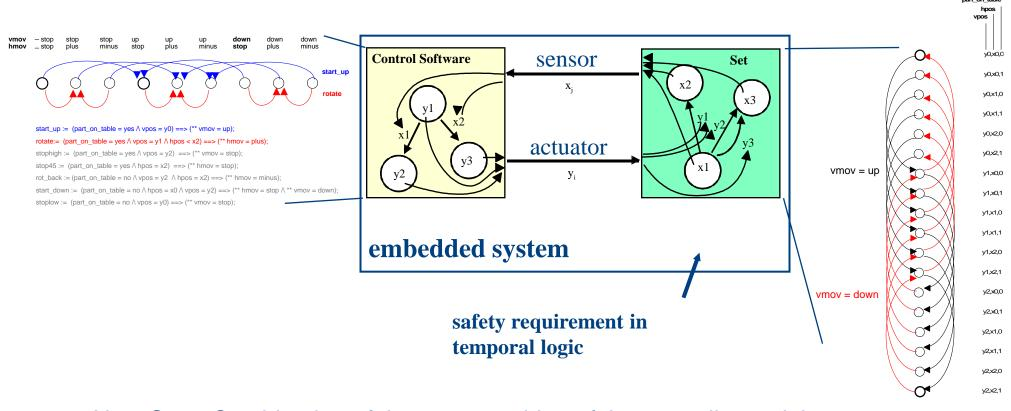
Next Step: Combination of the state machine of the controller and the state machine of the elevating rotary table to a so-called product fsm (finite state machine)
