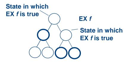
There has to be a directly following state in which *f* is fulfilled
