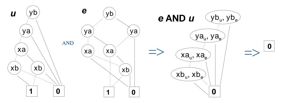
There are no reachable states that are unsafe, because the AND-operation applied to both sets of states produces the Boolean constant FALSE. The system is safe with regard to the defined safety requirement
