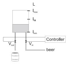
The system contains a sensor L that measures the beer-level in the tank. Its values are  $l_{min}$ ,  $l_{fill}$ , and  $l_{max}$ . The input valve  $V_{in}$  and the output valve  $V_{out}$  are actuators. The values are *open* and *closed*.
