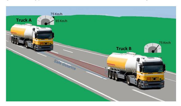
In the figure above we can observe that Truck B is going at a speed of 75 Km/h and Truck A is going at a speed of 85 Km/h. The ACC system installed in Truck A will reduce the speed accordingly (75 Km/h) so that a safe distance to Truck B is kept. Whenever there are no vehicles ahead Truck A, the system will return the speed to the initial value set by the driver (85 km/h). The ACC is composed out of the following modules:
