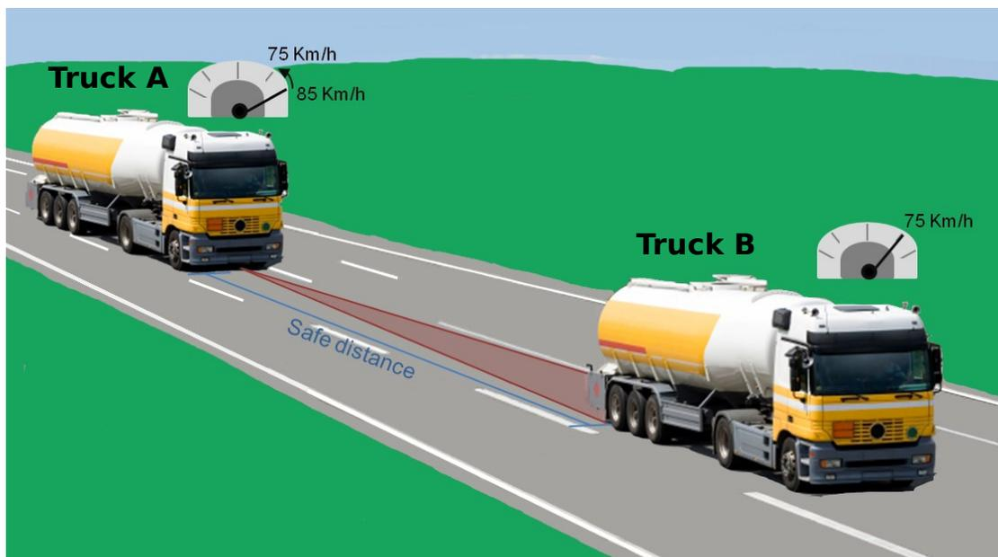
In the figure above we can observe that Truck B is going at a speed of 75 Km/h and Truck A is going at a speed of 85 Km/h. The ACC system installed in Truck A will reduce the speed accordingly (75 Km/h) so that a safe distance to Truck B is kept. Whenever there are no vehicles ahead Truck A, the system will return the speed to the initial value set by the driver (85 km/h). The ACC is composed out of the following modules:
